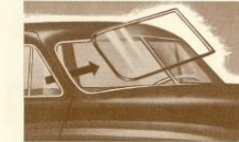
Safety Windshield —Laminated safety glass is mounted in sponge rubber interlayer to that a hard blow from within will split it in one piece. Thus, greatest collision hazard—lacerations or fractured skull from striking windshield—is entirely eliminated. Windows are armor plate glass which disintegrates without cutting edges or shivers.
