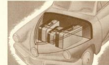
Safety Steel Bulkhead —A steel safety bulkhead surrounds the spacious luggage compartment located under the hood, thus shielding the passenger compartment from head-on collisions far more effectively than the conventional front engine construction. A second steel safety bulkhead walls off the rear engine.
