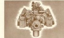
Rear Engine —166 horsepower, flat opposed six-cylinder engine located below the level of passengers. Aluminum alloy construction. More power for the weight of the car than any volume production automotive engine ever built. Eliminates fumes, heat, noise in passenger compartment.
