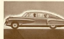
Frame Lower Than Center Line of Wheels —An exclusive feature made possible by locating engine in rear and eliminating conventional drive shaft. This, combined with Tucker suspension system, greatly reduces chances of skidding or overturning.
