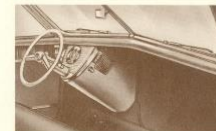
Crash Board Cowl and Safety Chamber —Conventional instrument panel is replaced by attractive sponge rubber crash board cowl. Instruments in steering column. Under cowl is spacious safety chamber, protected by steel bulkhead, which driver and front seat occupants can drop into, in a split second, in case of impending collision.
